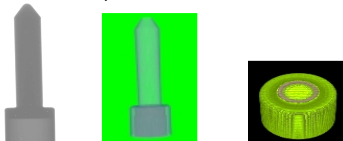
Fig. 2(a) Radiograph of MOX fuel end cap -Zircaloy (b) 3D reconstructed image (c) Cutway view of the weld
