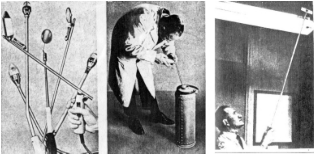
fig. 1 a) a collection of inspection mirrors. b) inspection of crevices and c) inspecting the inside of as cylinder
