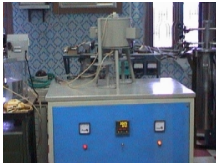
Fig.2. Experimental arrangement of the high temperature furnace for the ultrasonic velocities and attenuation measurements
