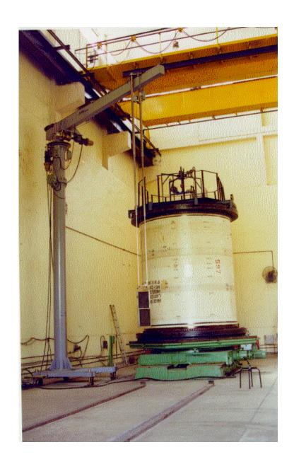
View of Radiography Film Positioning stand with PS1 Segment
