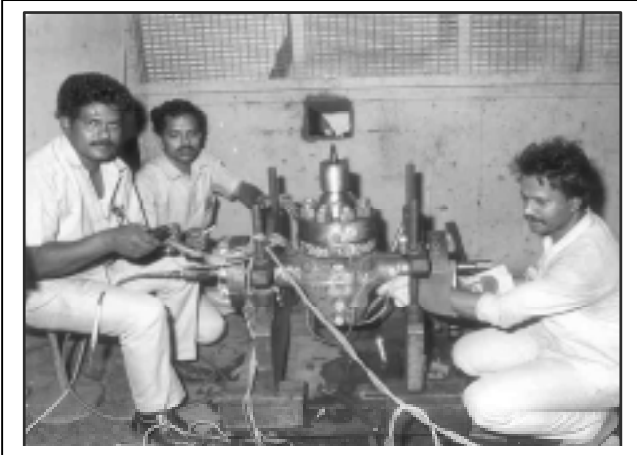
Fig 7. The strain gauge test for validation of the design of oil field equipment valve
