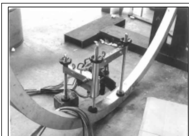
Fig 25 Residual stress measurements in ring rolled Al forgings
