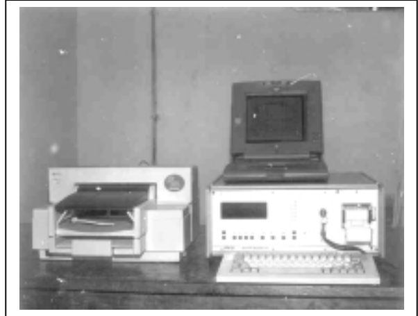
Fig 8. The digital strain meter used for strain measurements
