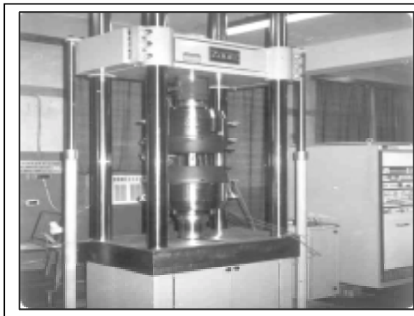
Fig 3. Calibration of the procedure with tensile testing machine
