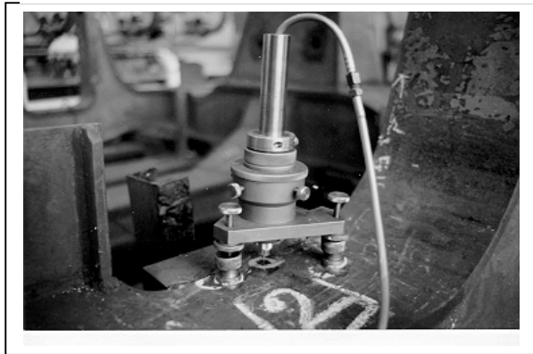
Fig 18 Blind hole drilling using high speed drilling mandrel
